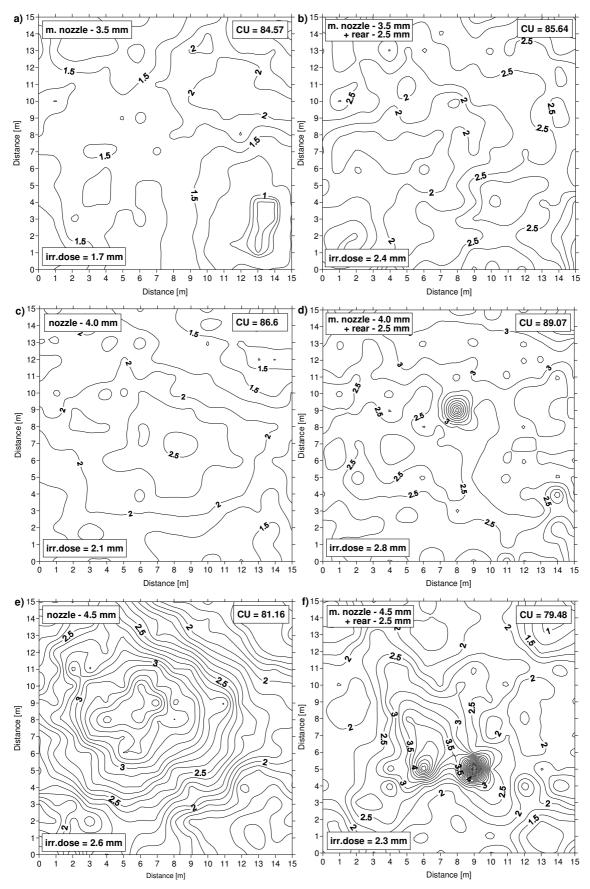
Fig. 2. Irrigation dose, Christiansen uniformity coefficient and irrigation dose distribution for sprinkler nozzles used in field experiments (part 1)
