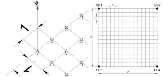
Fig. 1. Arrangement of catch-can pattern for four (SP1-SP4) sprinklers
