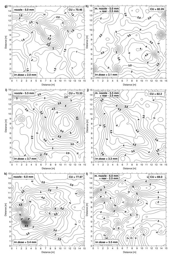
Fig. 3. Irrigation dose, Christiansen uniformity coefficient and irrigation dose distribution for sprinkler nozzles used in field experiments (part 2)
